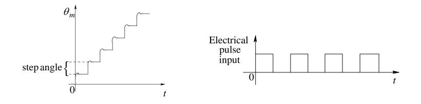
■ Each pulse moves motor a discrete angle – step angle
